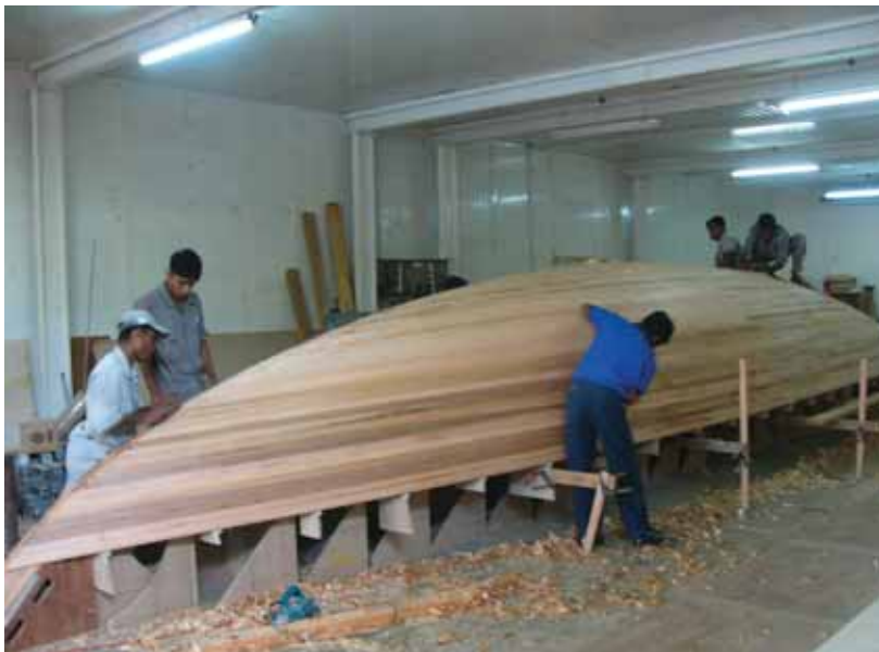
Fairing the cedar strip planking before glassing.
